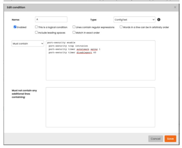
You can switch between condition types using the "This is a logical condition"-checkbox. Like policies, conditions can also be enabled or disabled. A disabled condition will not be evaluated from a rule's logic and compliance checks. Disabled conditions will also be greyed out in the conditions grid in the main compliance form.
