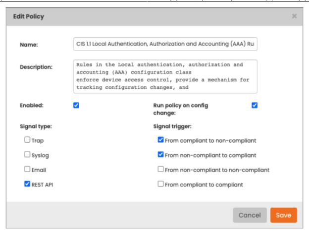
The options (Trap, Syslog, Email and REST API) presented under Signal type represent the available actions to be undertaken upon the compliance result. This can be triggered in four different ways:
