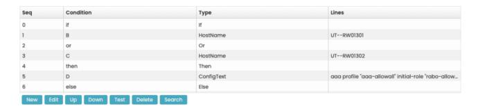
There are two types of conditions: Conditions that test a config block, and logic conditions that tie everything together. Logic conditions can be either 'if' ('then', 'else'), 'and', 'or' and '(' and ')' to group things together. Together they form a logic string that needs to be valid for a rule to be compliant. A rule won't work if the syntax of its conditions is invalid, you can use the 'test'-button at the rules-grid to verify this.
